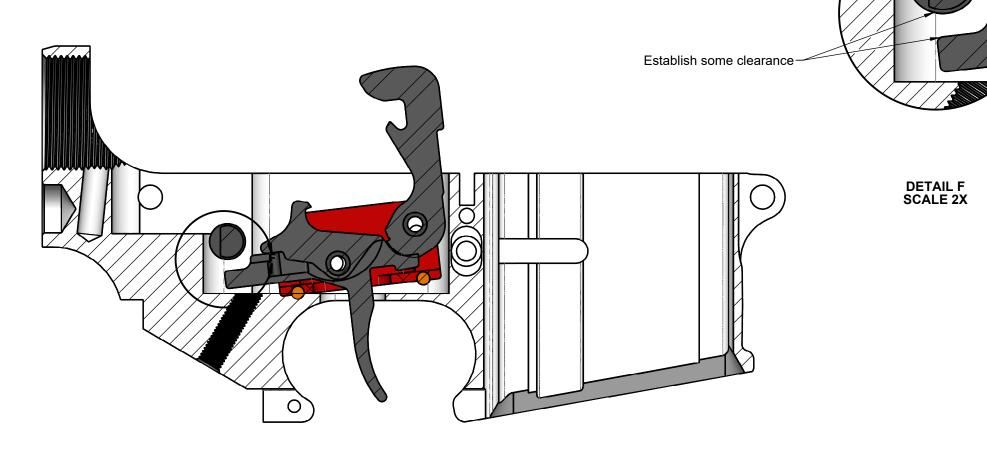
2a. Remove the Pistol Grip. With it should come the Selector Spring, and Selector Detent. This will allow the Selector to be moved at a later step.
